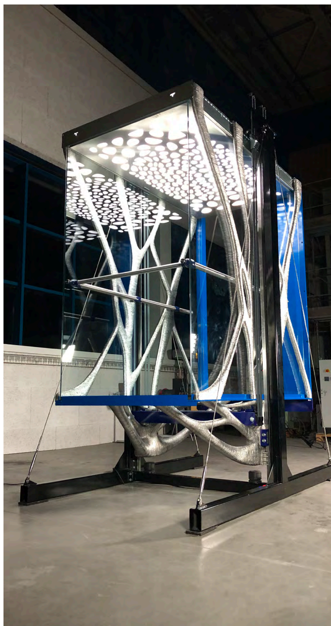
Assembled elevator car with standard car roof; courtesy of Schindler
